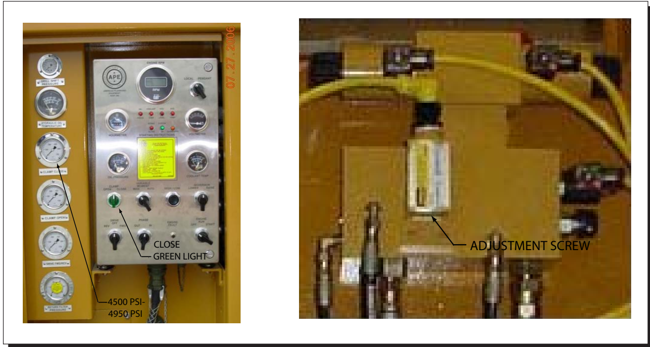
Figure 4-D. Checking Clamp Pressure Switch Setting
