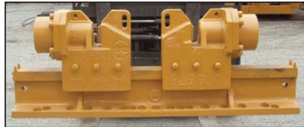
APE caisson beam & APE Model 200 caisson clamps.
