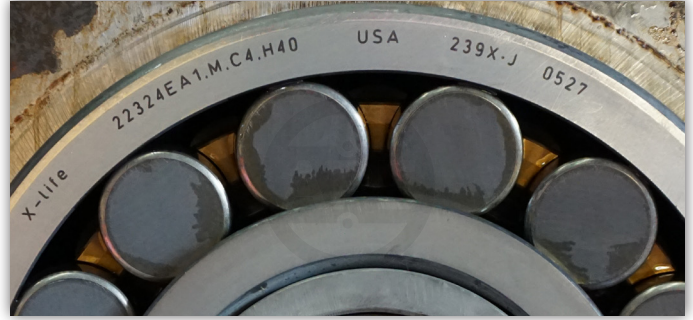
Etched words of manufacture location example: "USA" should be top center of bearings. If lettering is not on top, tap on the bearing with a rubber mallet to check if it is loose. Note: not all bearings are made in USA.
